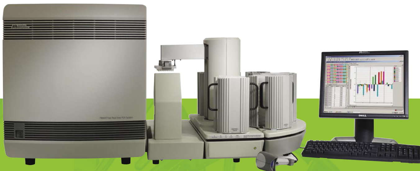
The Applied Biosystems 7900HT combined with TaqMan® Gene Expression Assays and the TaqMan® Low Density Array enables high-throughput and flexibility while streamlining reaction setup time.
